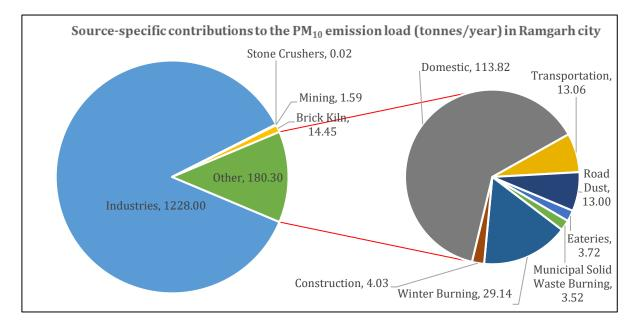
Figure 3: PM<sub>10</sub> emission load (tonnes/year) at the city level in 2019
